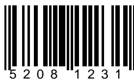
Fig. 6 : EAN 8 Symbol of the size SC5
