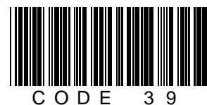
Fig. 11: Code 39 Symbol with the Information "CODE 39"
