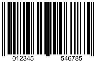
Fig. 3 : UPC - UPC-A Code with the information “01234554678” of the size SC5 (see Table 8)
